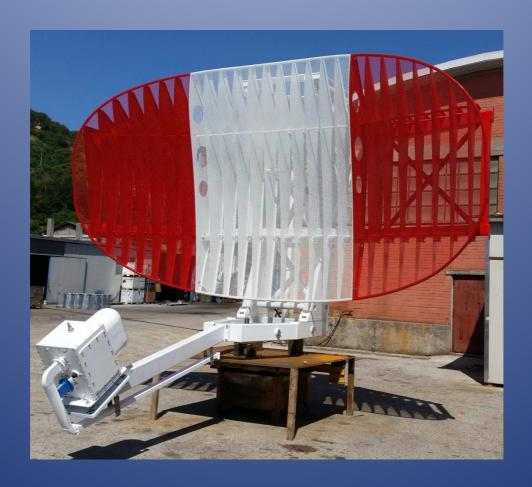
Approach (APP) Terminal Area (TMA) Primary Surveillance Radar Antenna Subsystem
